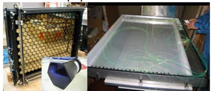
Fig 2: Camera of FD telescope (left) and inside of particle detector.
