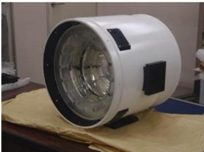
Figure 1 Acoustic lens of our acoustic imaging camera based on ultrasonic technology. The imaging camera can capture images underwater without light.
