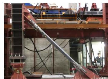
Fig. 1 Buckling-restrained braces
